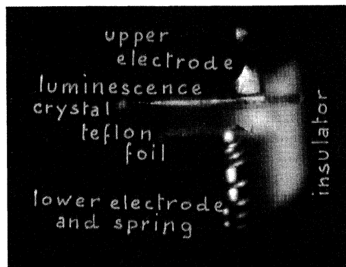
FIG. 3. Photograph of KI sample excited by an alternating electric field. Light emission is localized near the gold contact deposited on the upper face of the crystal. Applied field: 6 \times 10^4 V/cm. Frequency: 300 Hz.
